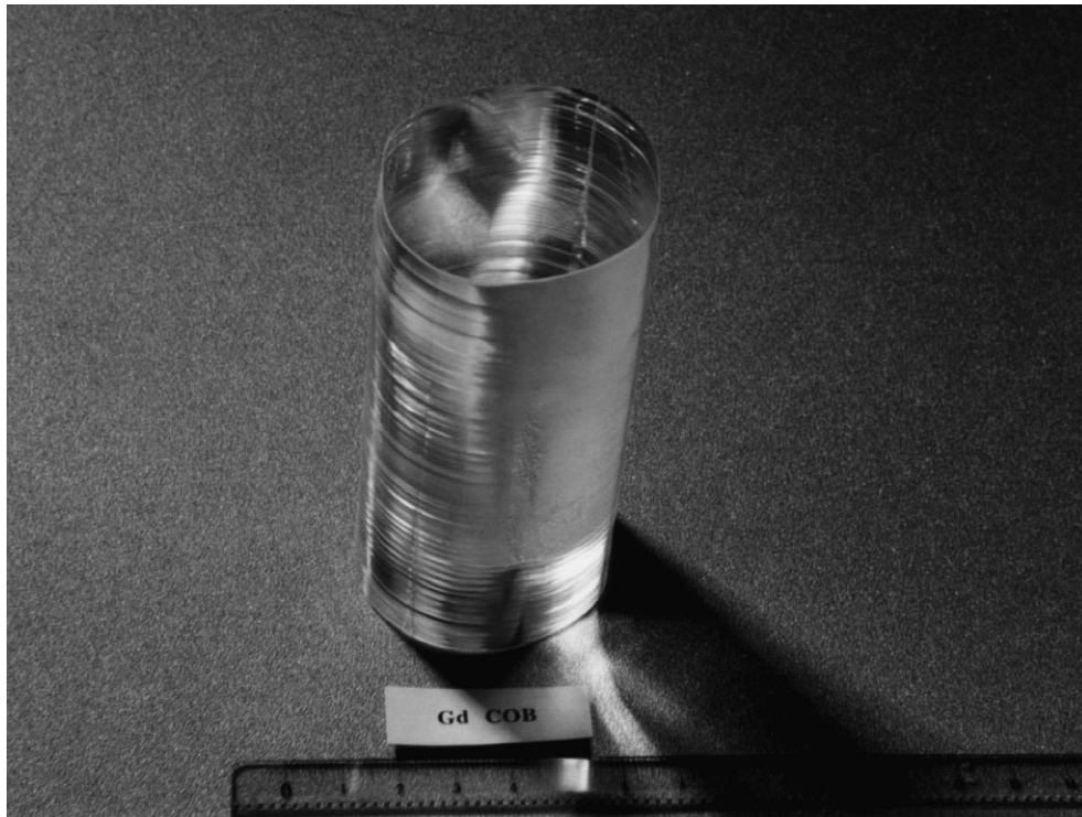
Fig. 2. A GdCOB single crystal grown from the melt by the Czochralski pulling method.
